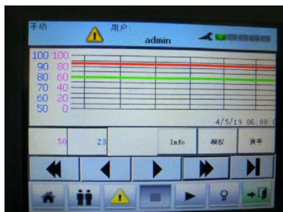
Test temperature and humidity curve
