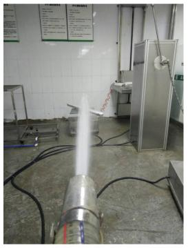
Photo 4: Test result after IP6X test and IPX6 test
