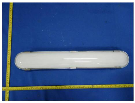
Photo 2: IP6X test of model FLT-TP-20L6
