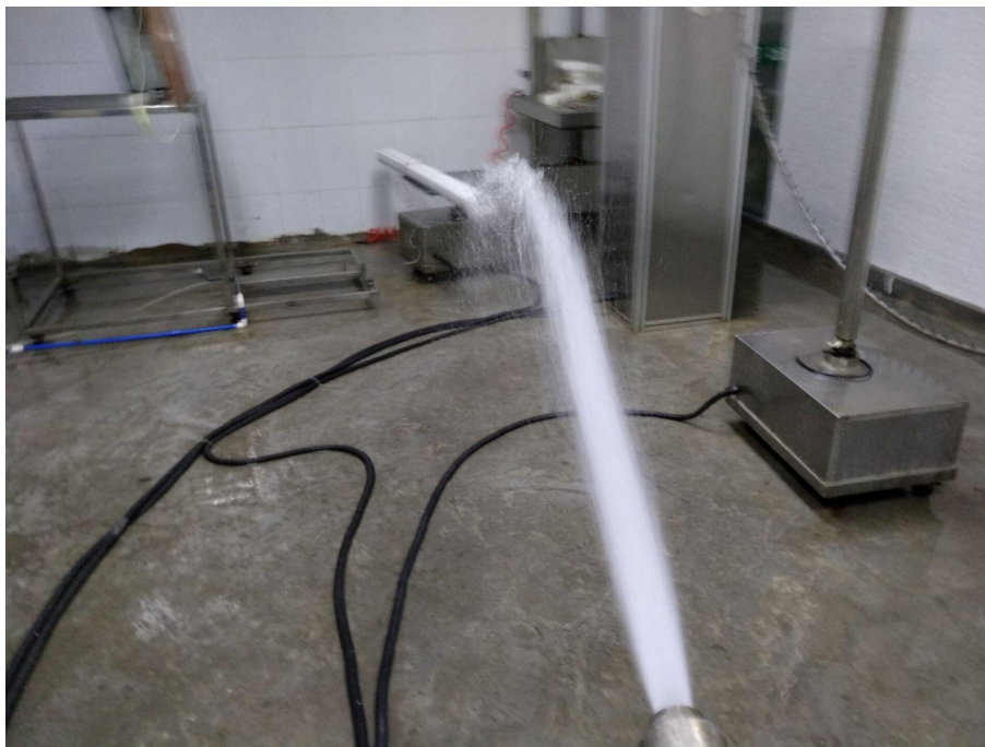
Photo 3: IPX6 test of model FLT-TP-80L15
