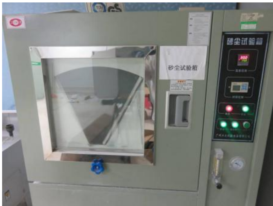
Photo 2: IP6X test of model FLT-TP-80L15
