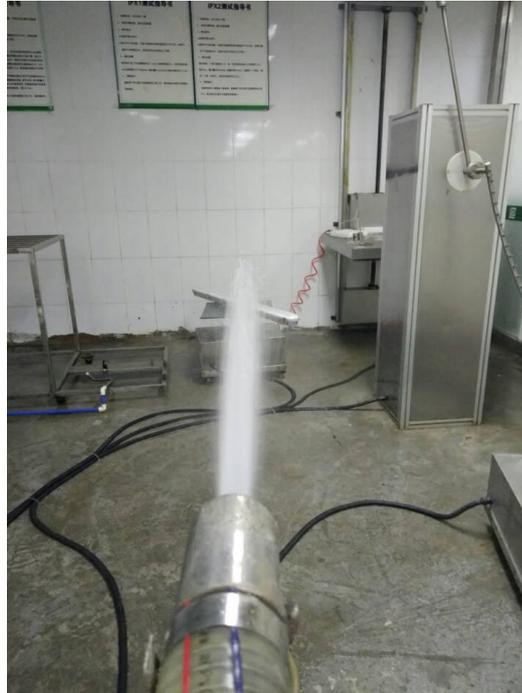
Photo 4: Test result after IP6X test and IPX6 test
