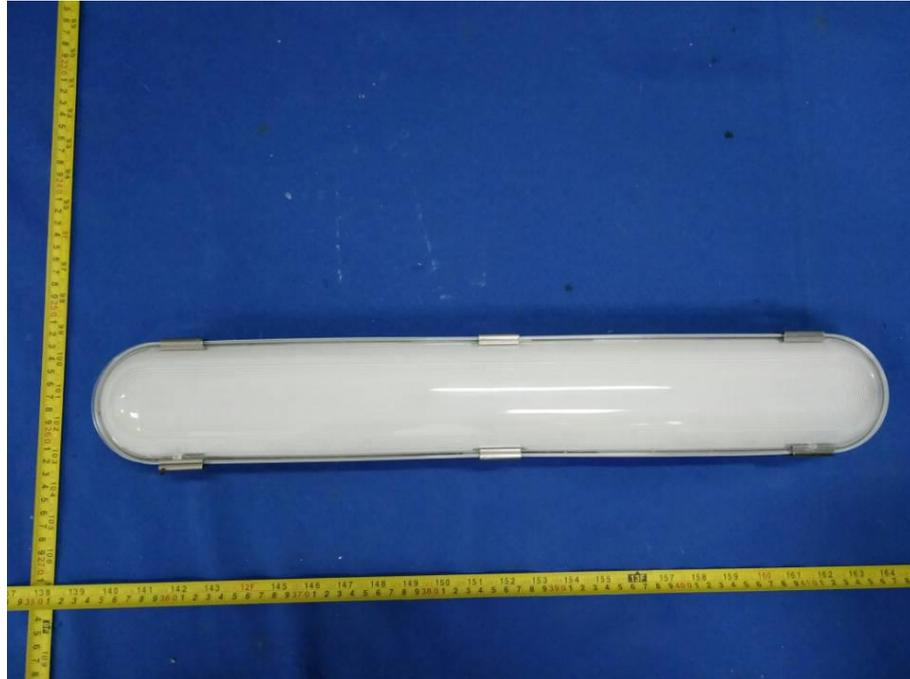
Photo 2: IP6X test of model FLT-TP-20L6
